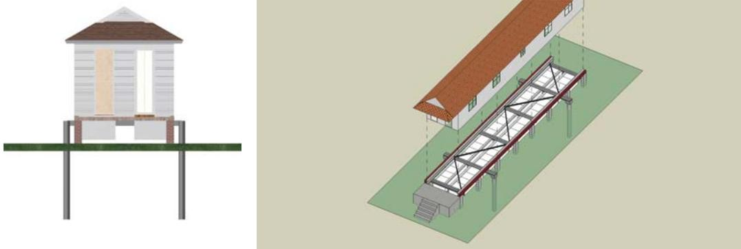
Figure 8: Schematic diagrams of the buoyant foundation system.
