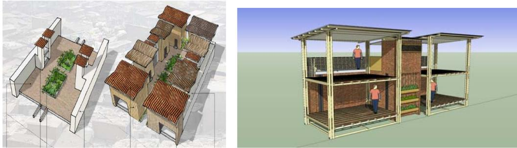
Figure 6: The LIFT House in Dhaka, Bangladesh. Eight-unit and two-unit clusters.
