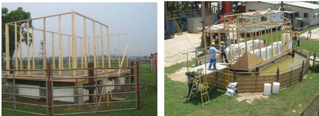
Figure 9: Full-scale testing of prototype buoyant foundation system. Construction of prototype; stability test showing floating platform tilted due to unevenly distributed sandbags representing imbalanced live load.
