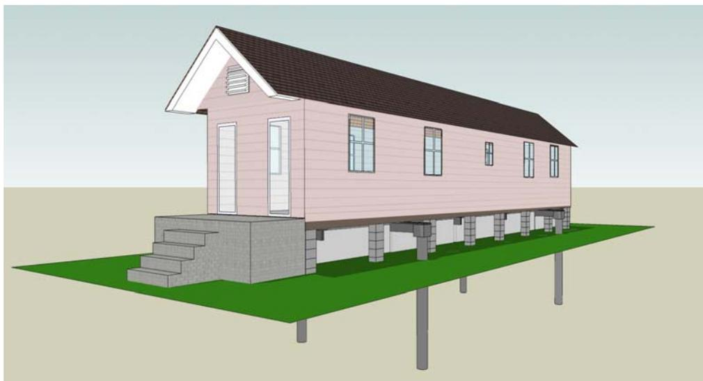
Figure 10: Rendering of a shotgun house retrofitted with buoyant foundation system.
