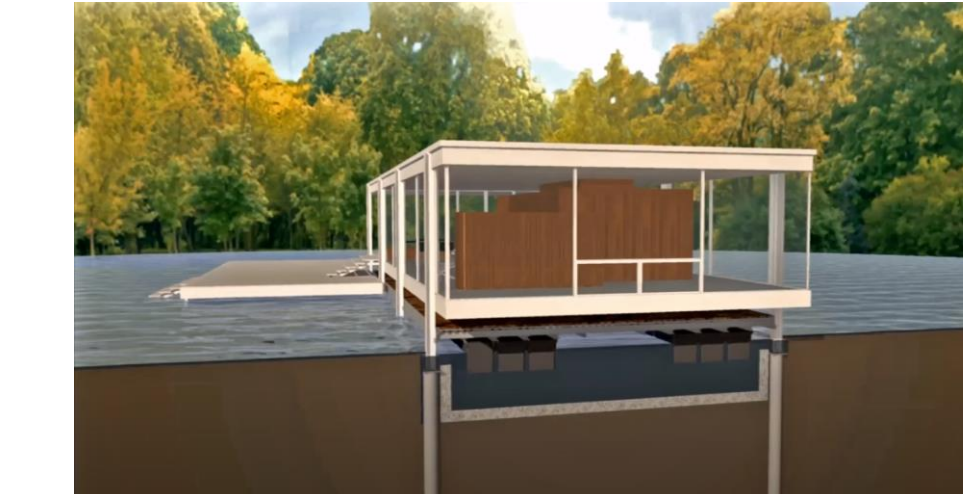
RENDER OF BUOYANCY SYSTEM
