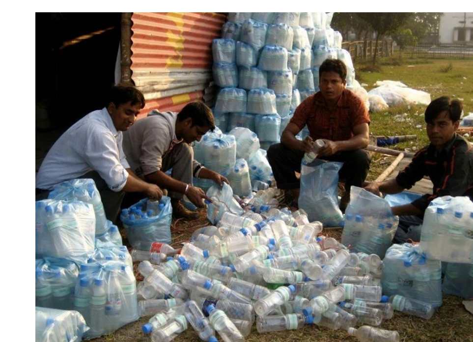
EMPTY PLASTIC BOTTLES BUNDLED INTO BUOYANCY ELEMENTS
