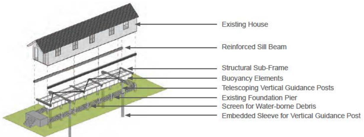
**Figure 4.** Components of a typical retrofitted buoyant foundation system
