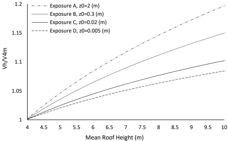
**Figure 5.** Ratio of mean roof height wind speed to 4m wind speed
