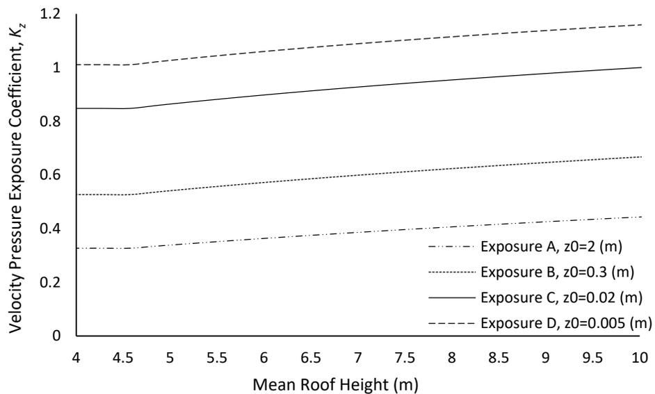
**Figure 6.** Velocity pressure exposure coefficient as a function of mean roof height
