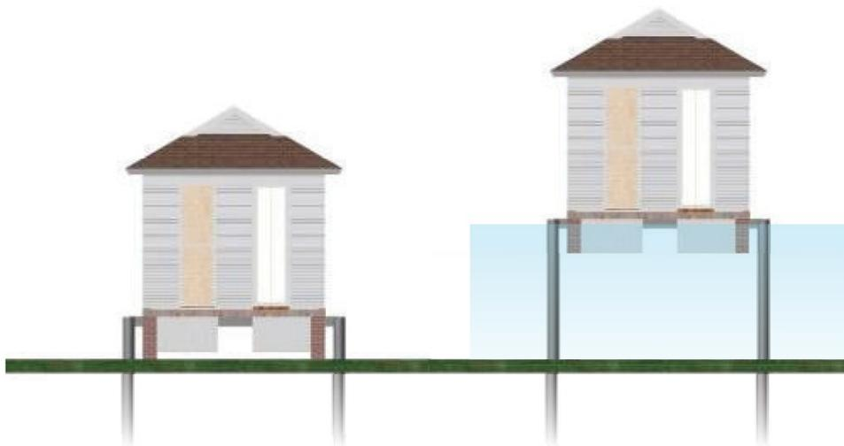
**Figure 2.** Schematic diagram of a buoyant foundation ([www.buoyantfoundation.org](http://www.buoyantfoundation.org))
